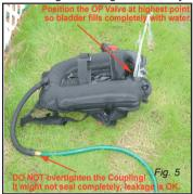
(OPV) and flow through the inner bladder flushing out salt and minerals. Pull both OPV strings occasionally. When the BC is flushed out, turn the water off and disconnect the garden hose from the coupling. Excess water can be drained out of the corrugated hose or from the Over Pressure Valves by pulling the release strings. DO NOT OVER TIGHTEN THE COUPLING. It is not designed to seal completely against a garden hose. A LITTLE LEAKAGE IS OK.
